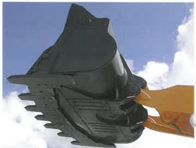
K VX teeth fitted to the bucket of the WA600.
