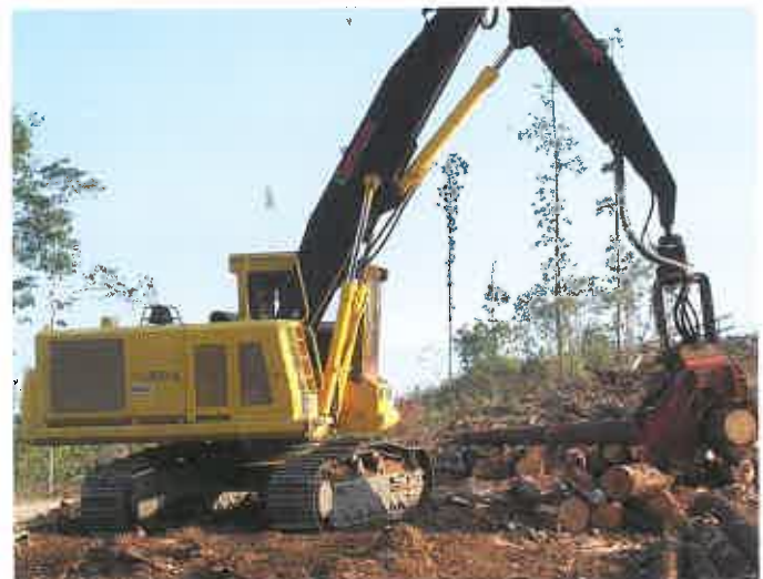
A PC300-6 excavator fitted with a Warratah Harvesting Head.
