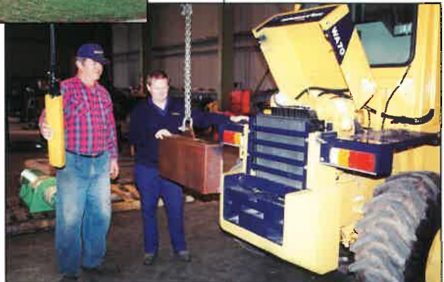
Neville Sandford and Bill Politis installing counterweight on a WA70-1 for BHP Ardrossan.
