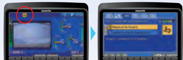
Aftertreatment device regeneration screen
