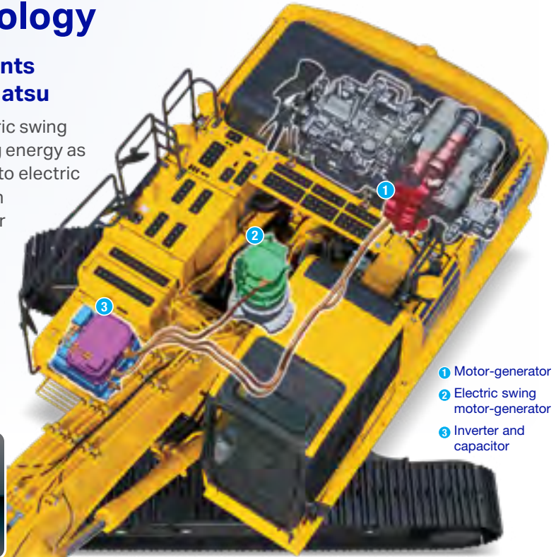
The upper structure swinging
