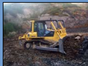
NZ’s Nightcaps Contracting operates a fleet of Komatsu excavators, plus a D65EX-12 dozer.
