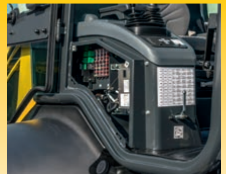
Side cover for quick maintenance access
