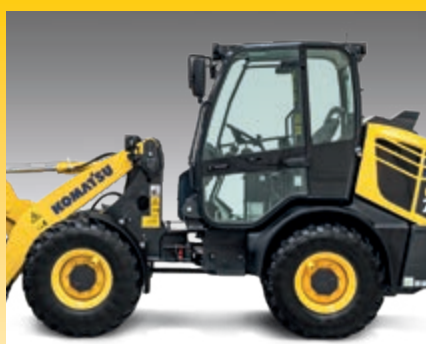
Low total height (2,48 m) for easy transport
