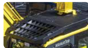
Bolt-on Top Guard OPG Level 2 (ISO 10262) for falling object protection.
