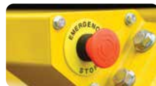
E-Stops Allow compliance to site safety requirements.
