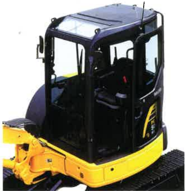
The cab on the new MRX-2 range is the same size as on a 20 tonne excavator and tilts up for easy access.
