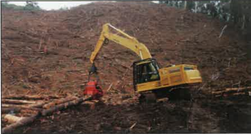
▲ PC300-6 owned by Cable Logging, Gippsland. This machine is fitted with a Waratah "Bigwood" processing head, the largest in Australia.
