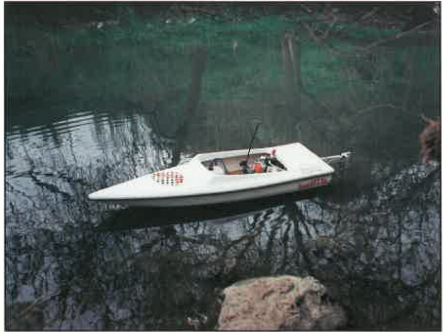
▲ 1/4 scale model racing boat, powered by a Komatsu Zenoah two-stroke engine.
