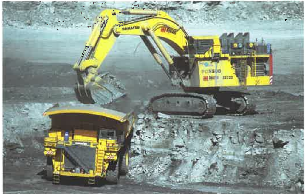
One of the PC5500's loading and 830E dump trucks at a Wambo mine site in the Hunter Valley.
