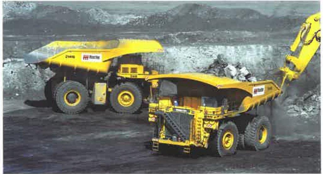
Two of Wambo's eight Komatsu 830E dump trucks being loaded by one of its PC5500s.
