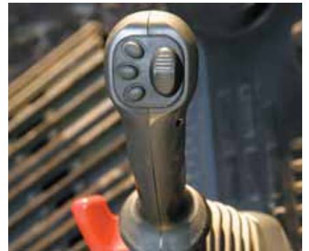
Joysticks with proportional control button for attachments
