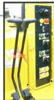
Upper Control Panel
