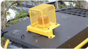
Rotating amber beacon Fitted with factory guard.
