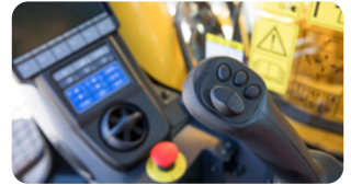
Proportional hand controls Enables proportional hand control of attachment speed.
