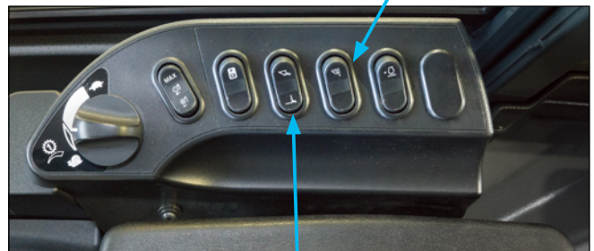
Attachment selector switch
