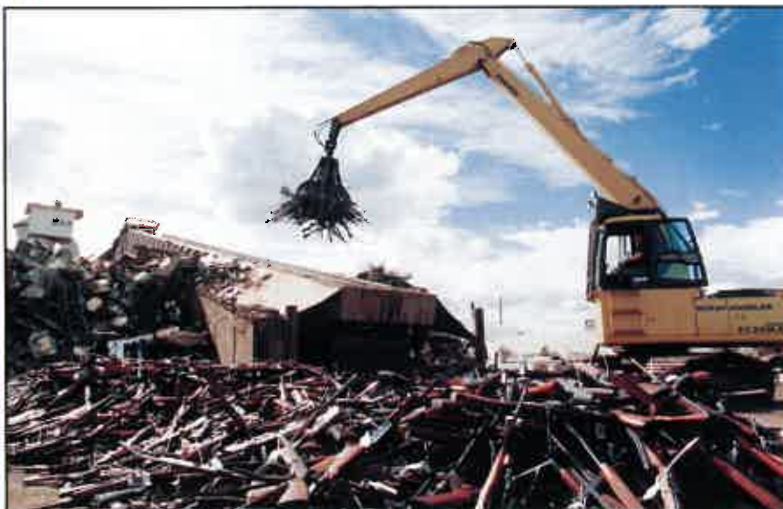
▼ Simsmetal Limited's PC250LC-6 Scrap Handler. Photo courtesy of Jerry Galea/ "The Age"
