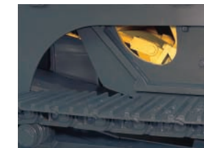
Opening In The Crusher Side (both sides of undercarriage)
