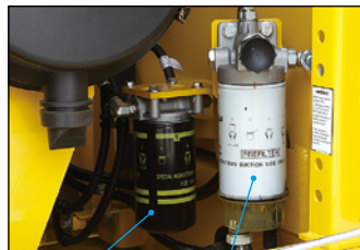
High efficiency fuel filter Fuel pre-filter (with water separator)
