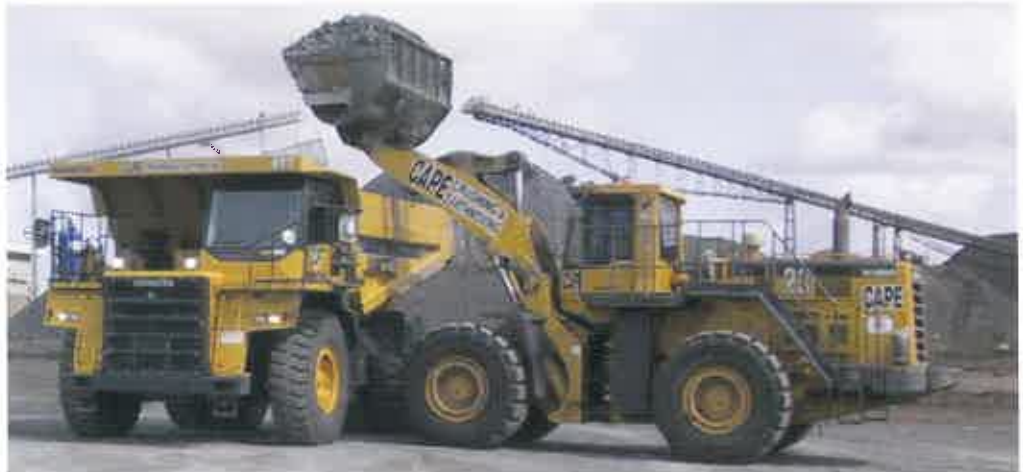
One of Cape Crushing's new HD465-7 dump trucks being loaded by its WA600-3 loader.
