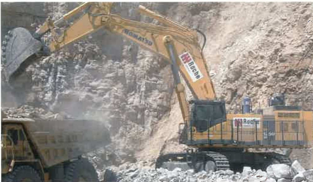
Roche Mining has standardised on PC1250-7 excavators for its contract mining operations around Australia
