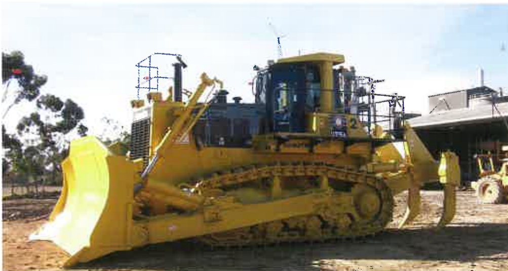
The new dozer features walkways and handrails around the cab and engine area for easier and safer maintenance.
