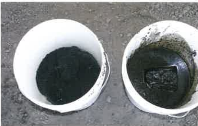
The bucket on the right is the original tarry mix; on right is the Reterra-processed material.
