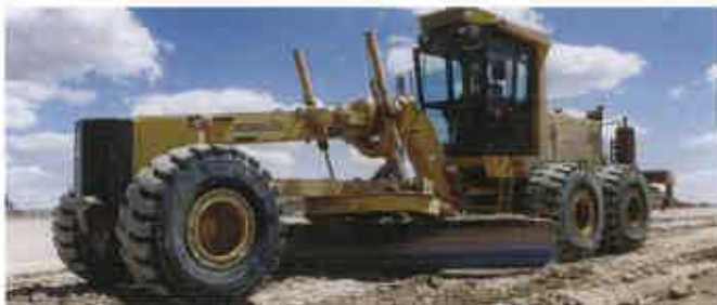
The GD825A-2 "Super" mining grader has been substantially beefed up and improved.
