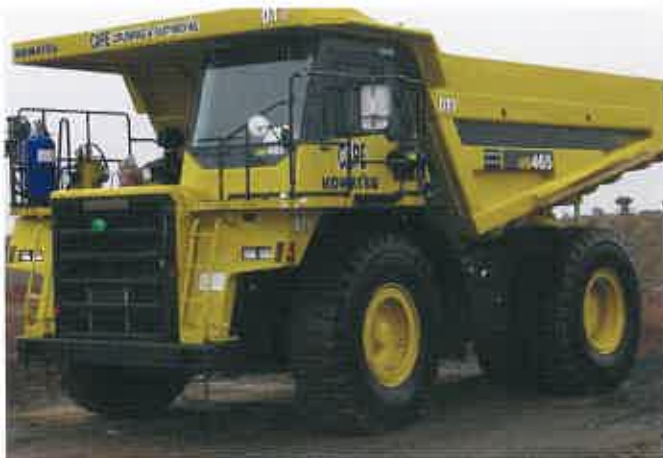
The addition of hungry boards raises capacity of the HD465-7s to 60 tonnes.
