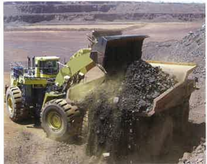
One of Pilbara Iron Yandicoogina's two WA1200s loading a 730E dump truck. A third WA1200 is due for delivery early next year.
