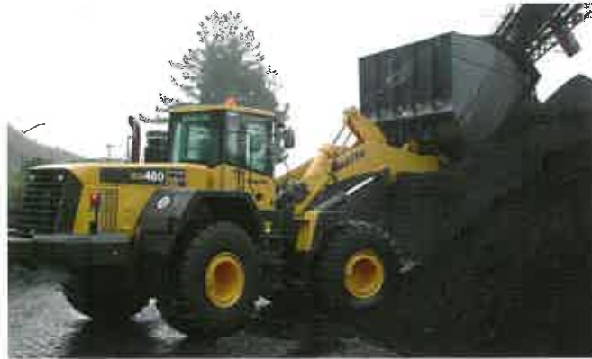
WA480-5 loader with an 8 cu m coal bucket at the Ngakawau Coal Facility.
