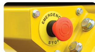
E-Stops Allow compliance to site safety requirements.
