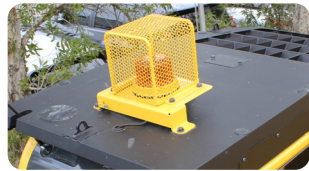
Rotating amber beacon Fitted with factory guard.
