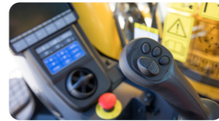
Proportional hand controls Enables proportional hand control of attachment speed.
