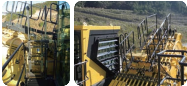
Access to boom catwalk
