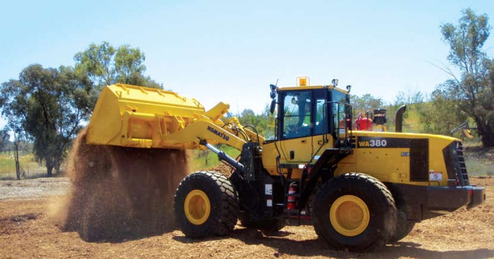
Pictured Above: WA380-6H wheel loader is used for bark handling, fitted with conventional sized 3cu m bucket. Right Inset: WA380-6H is the second wheel loader used for handling waste paper in the paper recycling operations.
