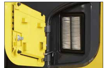
External air conditioner filter
