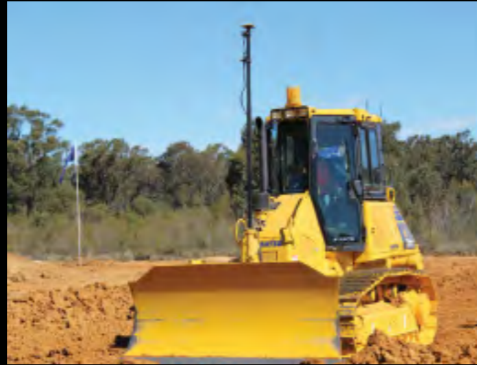
Komatsu's D51-EX22 fitted with Topcon's GPS Machine Control (3D) System
