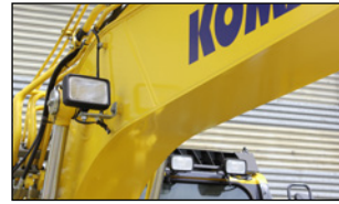
Additional Lighting Extra lighting on cab and counterweight for improved visibility.
