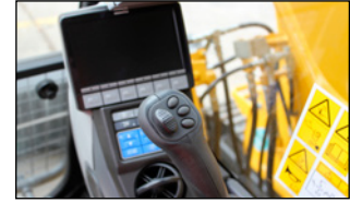
Proportional Hand Controls Enables proportional hand control of attachment speed.
