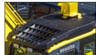
Bolt-on Top Guard OPG level 2 (ISO 10262) for falling object protection.
