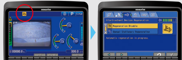
Aftertreatment device regeneration screen
