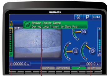
Ecology gauge Fuel consumption gauge Ecology guidance
