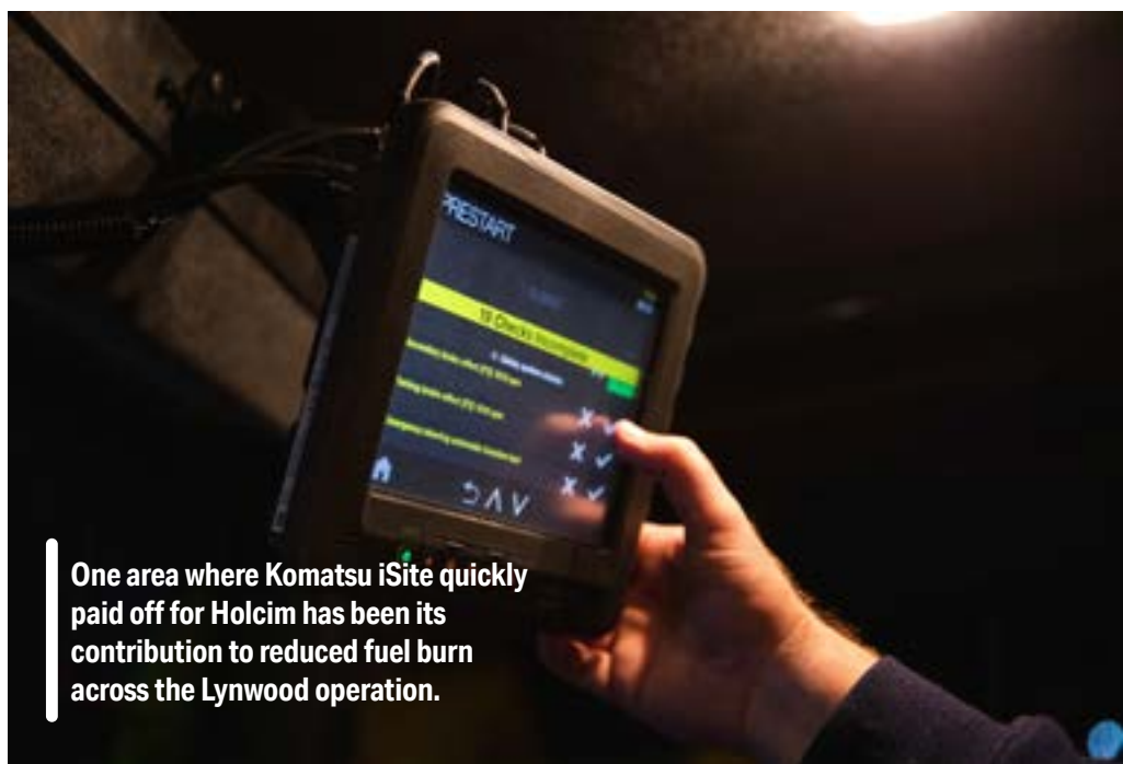
Pictured above: Operator using the in-cabin screen XD8 conducting electronic prestart.
