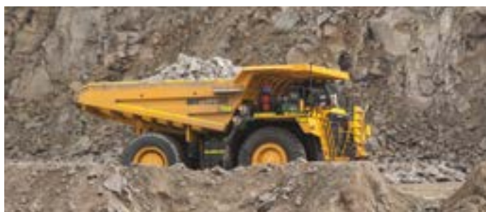
Pictured above: HD785-7E0 Rigid Truck with a full load hauling a productive load up the man haul road to the primary crusher.
