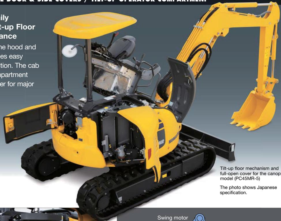
Tilt-up floor mechanism and full-open cover for the canopy model (PC45MR-5)
