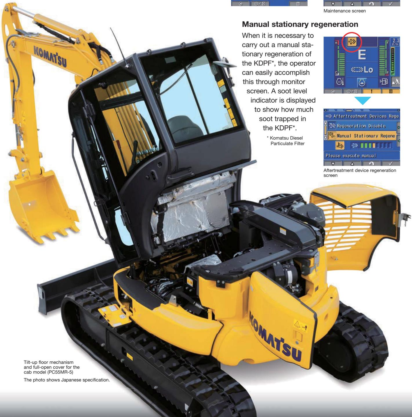
Tilt-up floor mechanism and full-open cover for the cab model (PC55MR-5)
