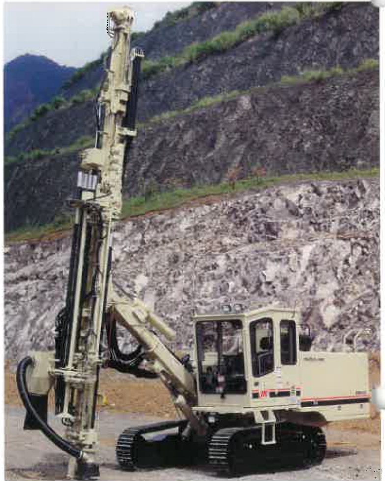
Below: Ingersoll-Rand ECM-660 Hydraulic Crawler Drill
