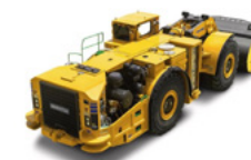
LHDs (load, haul, dump machines)
